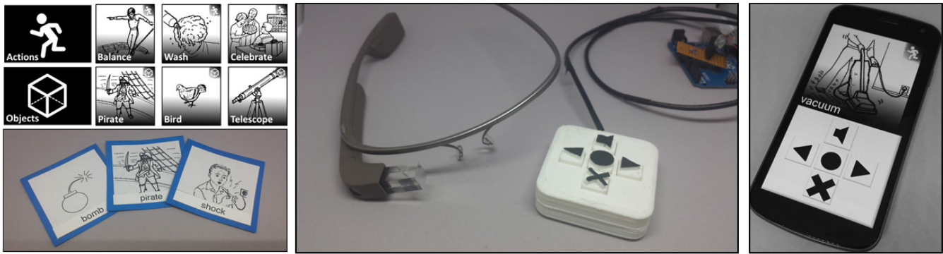
Figure 2. Top-left: Words from the vocabulary-prompting software, showing both the top level of the hierarchy (‘actions’ and ‘objects’) and examples of words from the second level. Bottom-left: Examples of Go Fish cards used for introducing the game; card sets used for the training and testing tasks were identical except they did NOT include text. Middle: HWD with remote control for navigation: cycle through words in the current level of the hierarchy (left/right arrows), select a top-level category and view its contents (circle), cancel out of the second level and return to the top level (‘X’), and play audio for the current word (speaker icon). Right: Smartphone version, showing an action word above the navigational controls.
